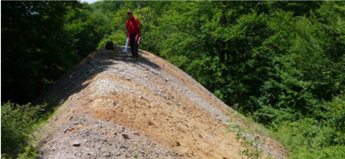
Figure 3: Mullock dump from an exploration gallery driven into Vein 10.
